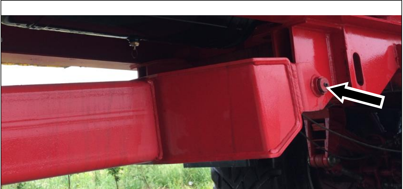
Figure 47: Lubricating nipple on the draw gear (same on the left and right)
