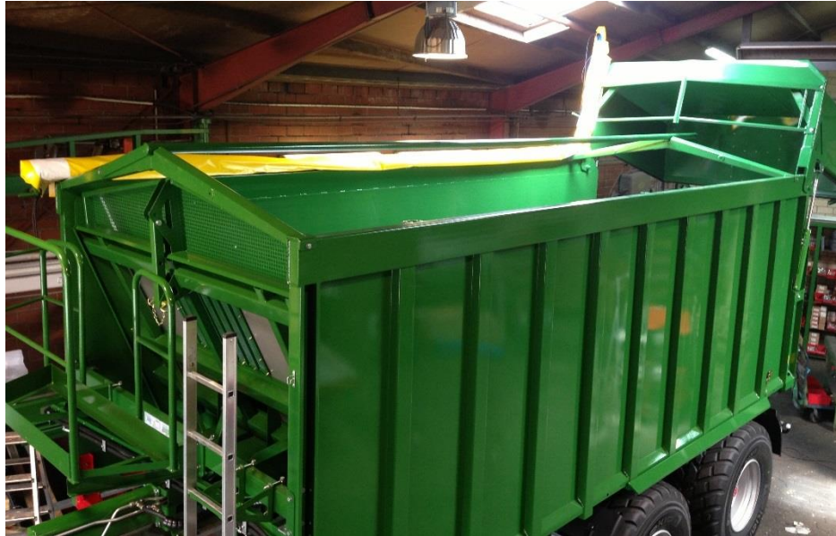
Figure 41: Roller tarpaulin open and secured
