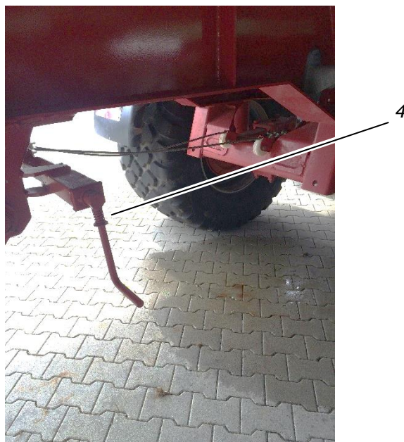
Figure 27: Parking brake (crank in adjustment position), here: TAW 20
