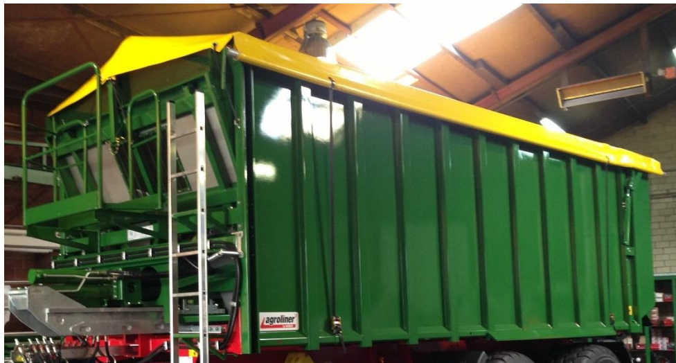
Figure 40: Roller tarpaulin closed correctly
