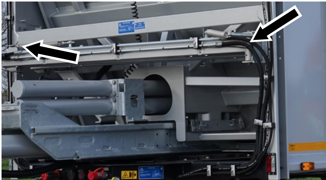
Figure 50: Lubricating the pipe support
