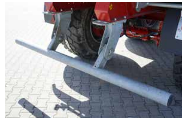
Mechanical foldable underride protection
