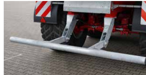
Hydraulic foldable underride protection
